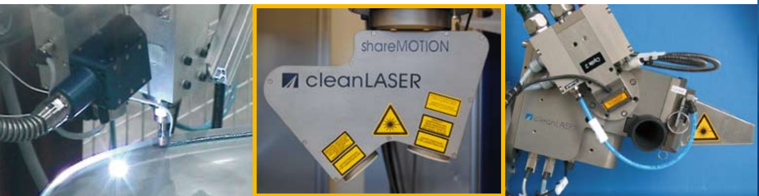
Optic for simultaneous bonding pre-treatment with integrated adhesive application
